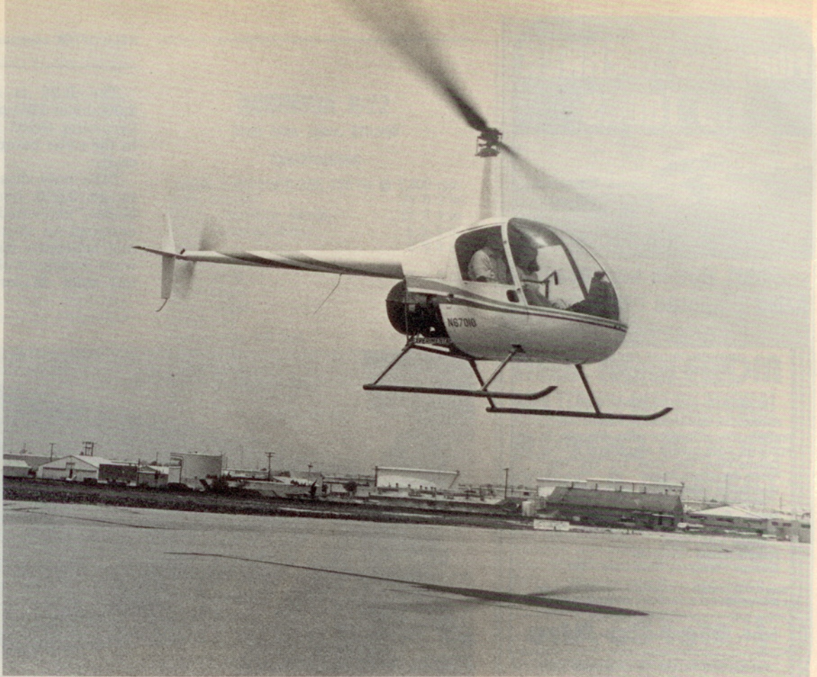
Robinson R-22 aims to compete in price range of four-place lightplanes, carries two at 100-mph cruise speed.
